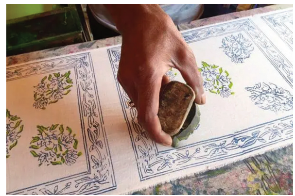
Block printing process
