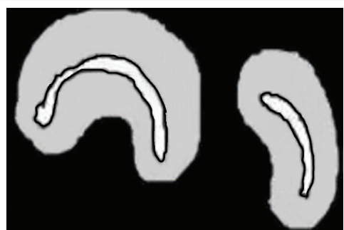
Cross-section of cotton fibres
